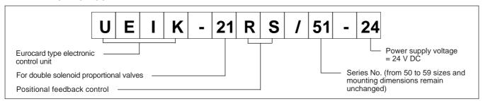
The UEIK-21RS card is an electronic control unit Eurocard type for closed loop control of double solenoid proportional valves with positional feedback control.
